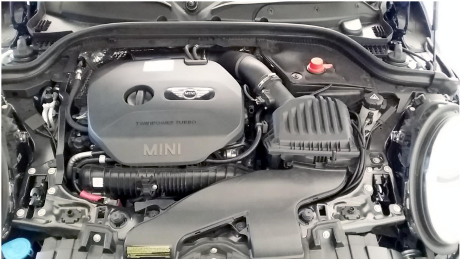
Before starting installation open the hood, close the doors, lock the vehicle, and let it sit 5 minutes for the DME to go to sleep. Place the keys inside so you don't accidentally wake it up during the install process.
