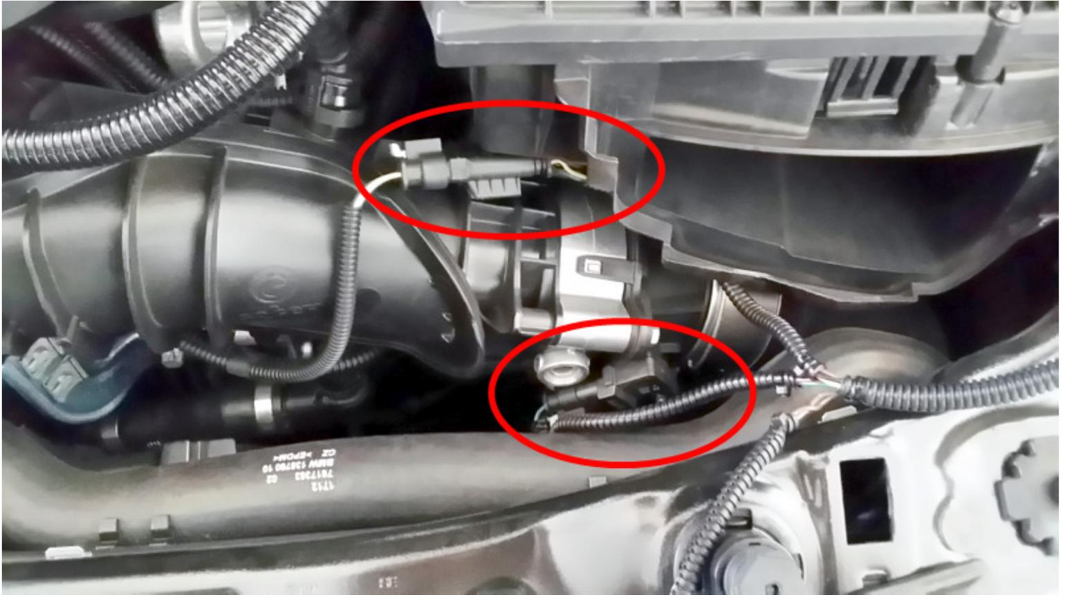
5) Route the harness towards the driver side as shown and reinstall the air duct removed in the first step.
