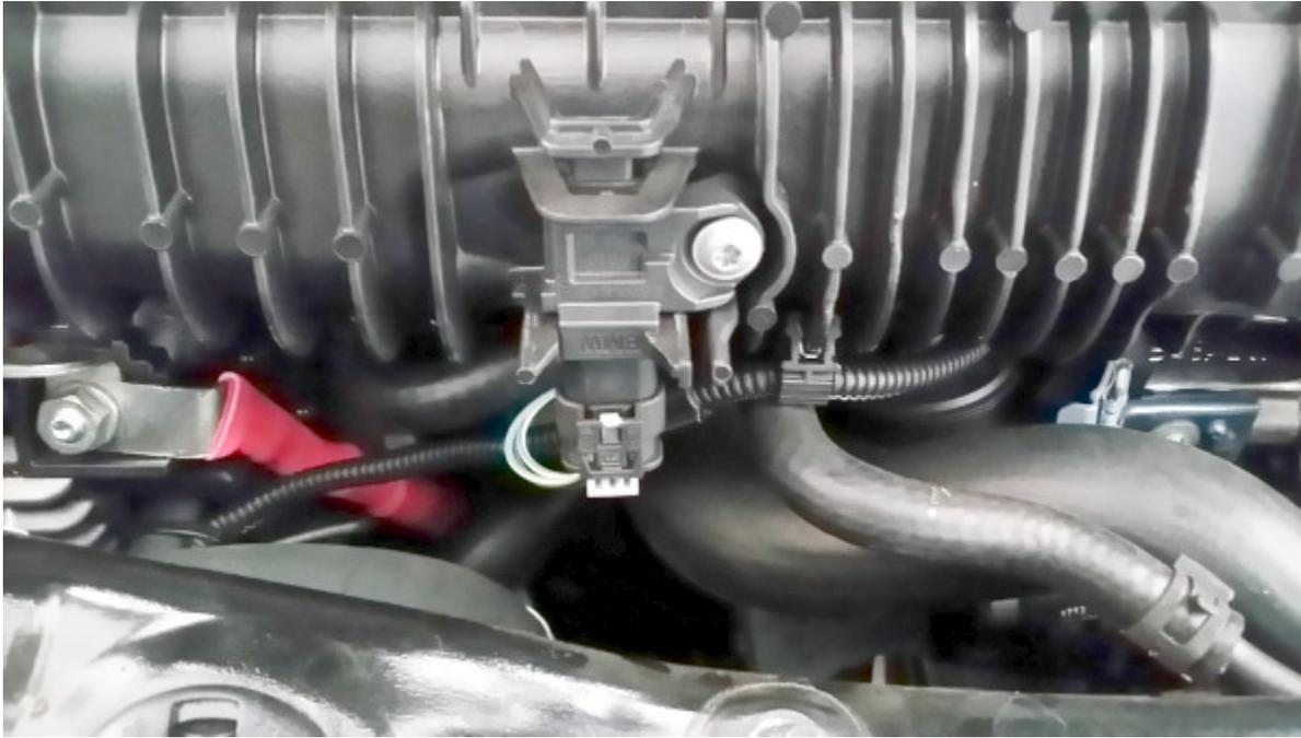
3) Plug the JB4 brown patch in to the sensor and plug the OEM connector in to the remaining connector on the brown patch.
