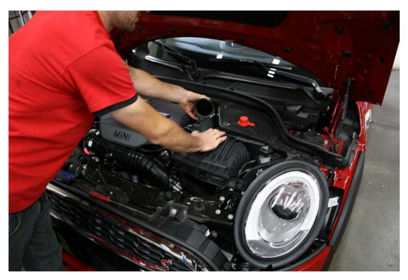
8. Separate the intake filter housing from the intake hose. Again, this will probably take some elbow grease.
