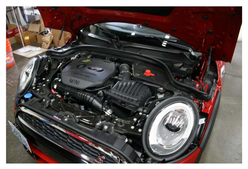
4. Remove the ducting. You'll need to finagle it apart from the intake filter housing. This part is also known as the "Intake Muffler", so get ready to make some noise!
