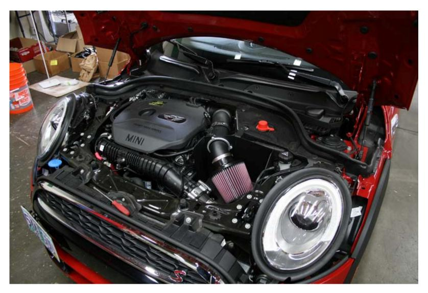
13. Rotate the filter, intake pipe and MAF housing so that the filter angled down into the air box at about 45 degrees (as shown). Place the entire assembly in the cavity left when you ripped out the stock lung.
