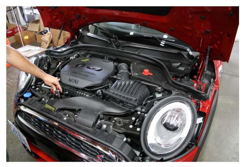
3. Remove the two 10mm bolts holding the air ducting in place.
