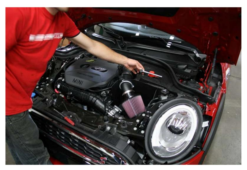
14. Replace the bolt from the top of the battery box, this time through the restraining tab of your new intake box.
