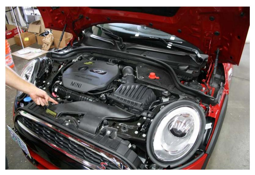
2. The first order of business is to get the air ducting out of the way. To find the intake duct, follow the magic finger in the illustration.
