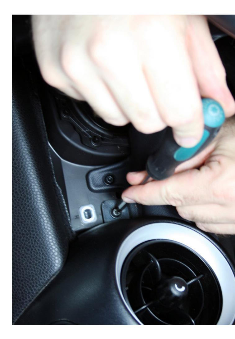
The next step most difficult part of the installation, removing the screw from the top of the vent cover. It is at an odd angle and very difficult to get to. We used a very small Torx bit on a little ratchet driver. Once the screw is out, the whole cover piece will slide right off.
