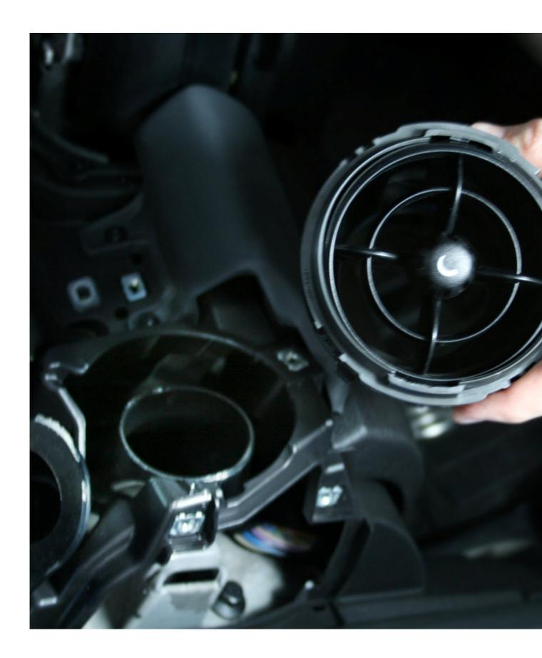
With the plastic pry bar, remove the plastic ring that holds the vent assembly together.
