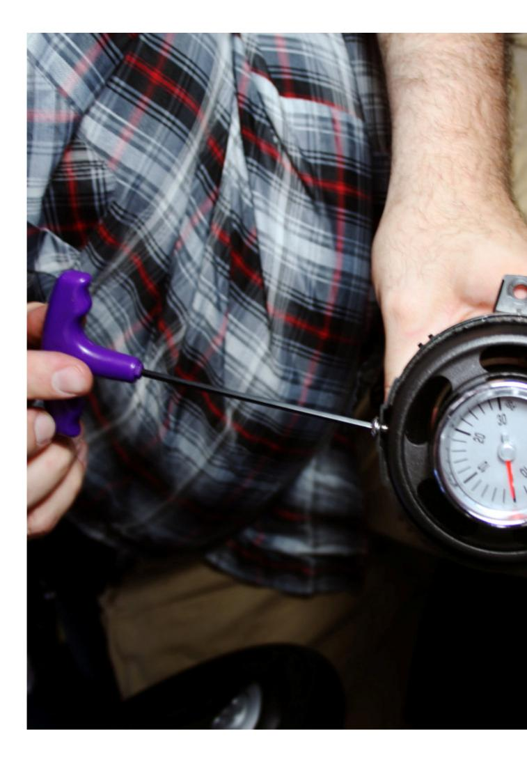
Now it is time to put the vent assembly back on your MINI. There will be enough room to run the gauge wires between where the vent assembly connects to the vent tube. Hold onto the wires and slide the assembly onto the tube. Twist the assembly to the left so it clips in and re-install the screw at the bottom.
