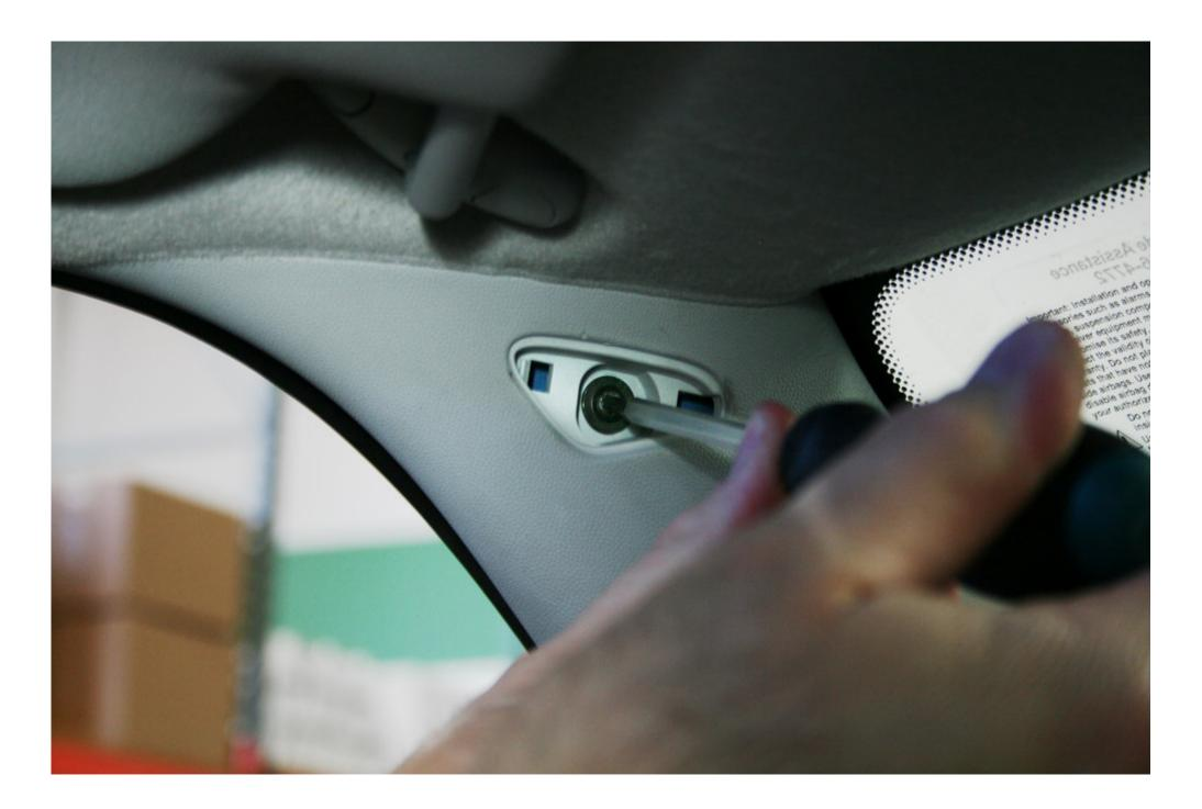
Pull the A-Pillar towards the center of the car and then towards the back. It is held in by clips.
