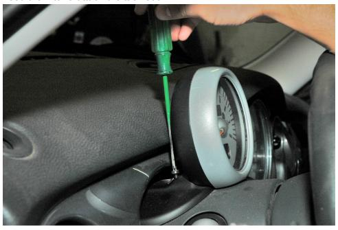
Lean the face of the Tach down toward the steering column giving you a view remove the top and left (left as you face the back of the tachometer from the drivers seat) screws from the tach. You will not need these screws for this installation, but if you want to keep the Fixie for your next MINI and return this one to stock, you will want to save them.
